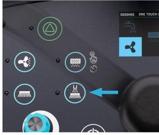
**11.** Turn DustGuard<sup>™</sup> on and off as needed. DustGuard<sup>™</sup> provides a light water mist to reduce airborne dust.
