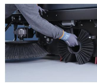
**20.** Remove, clean and inspect the main broom and check the side brooms. Clean the machine with a wet cloth.
