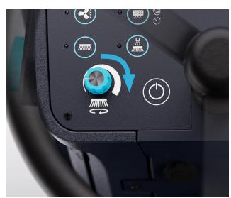
**10.** Adjust the speed of the side brooms by changing the side broom speed knob.
