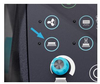
**16.** Press the side broom button to lift the side brooms and use the machine with only main broom.
