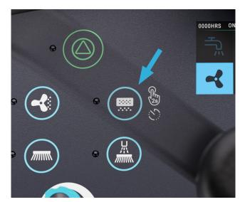
3. Clean the panel filter by pressing the filter shaker button.
