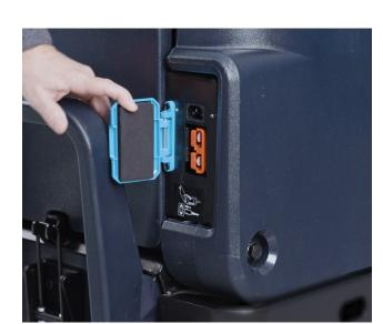
21. Charge the machine using the rear charging connection. It has two connections, one for external charger and one if on-board charger is installed.
