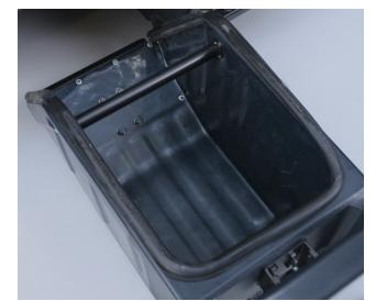
4. Check to see if the debris hopper is full or the hopper gasket is damage.
