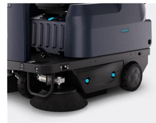
**3.** Ensure the main broom and side brooms are properly installed.
