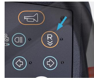
**15.** Press the reverse button to move the sweeper backwards. Machine does not sweep in reverse.
