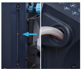
2. Check the solution level on the side of the machine. Add fresh water as needed by removing the blue cap on the fill port.
