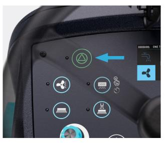
**7.** Press the start button to activate cleaning functions.
