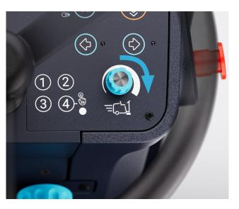
**9.** Turn the speed knob to adjust and set maximum speed with full pressed drive pedal.
