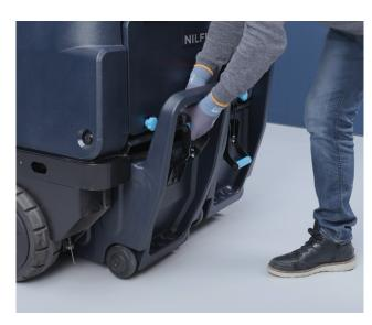
**18.** Press the OneTouch™ button to stop all functions. Slowly release the hopper locking mechanism as it may be heavy. Use the handle to remove and empty the hopper.
