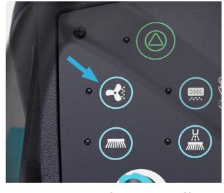
**17.** Turn the dust fan on and off as needed or when sweeping minor wet debris.
