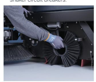
1. Inspect the main broom, make sure it's turning and is not worn out. Adjust broom pressure by the blue knob on the steering column if needed.
