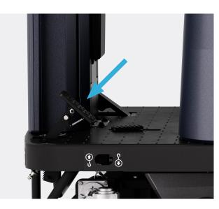
**12.** Press the front flap pedal to open the front flap for sweeping larger debris.
