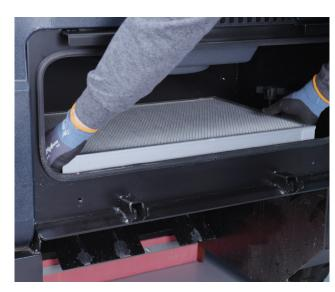
**19.** Remove the rear filter panel to check the filter, reinstall panel and hopper.
