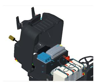
5. Open machine cover and disconnect the battery cable check so no fuses have tripped.
