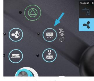
**13.** Use the filter shaker as needed. Press and hold to automatically activate every 10 minutes
