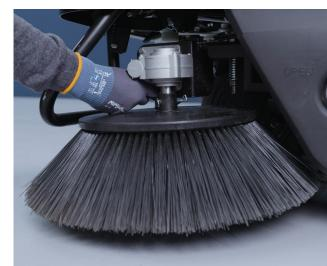
2. Adjust the side broom if needed, replace the side broom if bristles are worn out.
