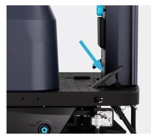
**8.** The brushes and vacuum will start when the drive pedal is pressed, start sweeping.
