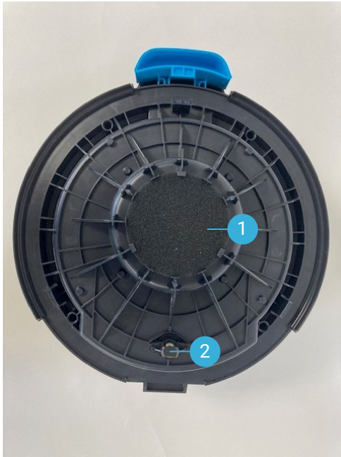
1 Filter 2 Vacuum valve. Valve ensures cooling for the turbine if the bendend/hose/bag is blocked
