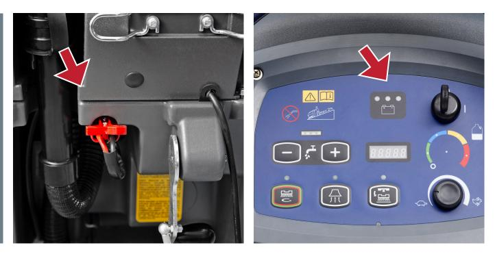
Check if the power cable is correctly 2 Check if the battery is charged.
