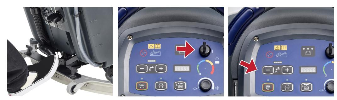
6. Lower the brush deck with the pedal. 7. Turn on the key, then slightly press the handle switch to engage the brush.
