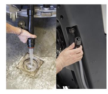
10. Once you have finished cleaning empty the recovery tank with the hose. Then empty the solution tank with the trasparent hose.
