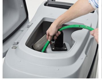
11. Wash with clean water the recovery tank and the vacuum grid.
