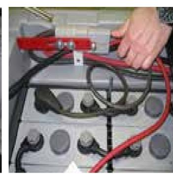
3 Check battery cables are well connected together.
