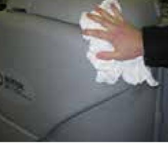
19. Clean the machine using a damp cloth and park it with the recovery tank open
