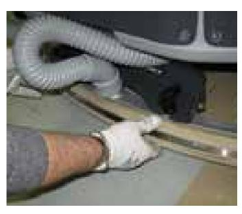
4. Connect the vacuum hose to the squeegee and then fasten it to its assembly
