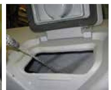
2. Fill-in the tank with clean water. In case hot water is used, this must not exceed 40 °C
