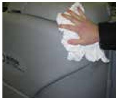
19. Clean the machine using a damp cloth and park it with the recovery tank open
