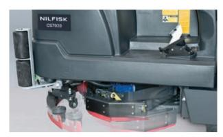
Retractable 10 cm offset disc deck enhances edge scrubbing and resists damage from accidental impact.
