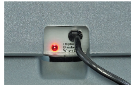
Carbon brush indicator lights red when brushes need to be replaced.
